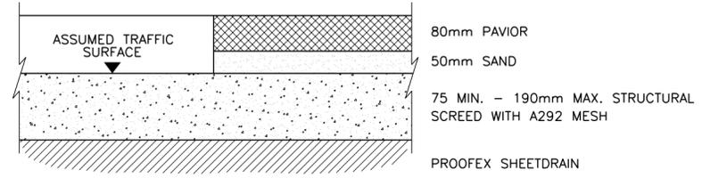
COVER ABOVE SHEET DRAIN TO FINISHED ROAD LEVEL LESS THAN 320mm
